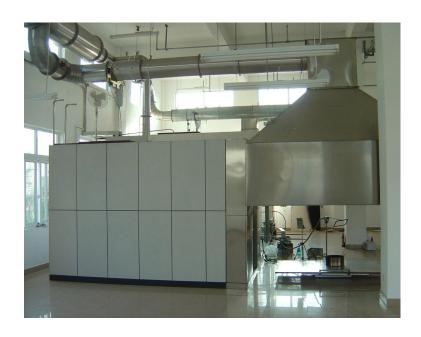
This apparatus is designed according to GB/T 34441-2017, it can test combustion performance of soft furniture mattress exposed to flame ignition source.
